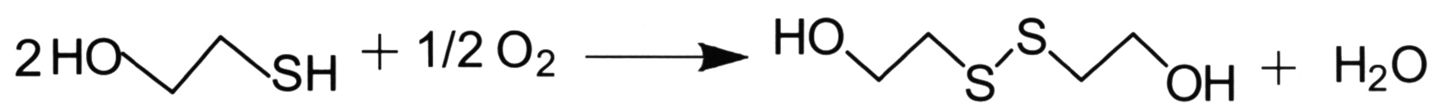
Scheme 3 Scheme of the oxidation of 2-mercaptoethanol.
